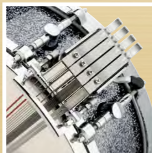
Master switch to engage / disengage simultaneously
